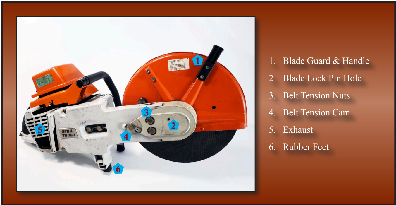
Figure 5-11 Right Side Rescue Saw Schematic
