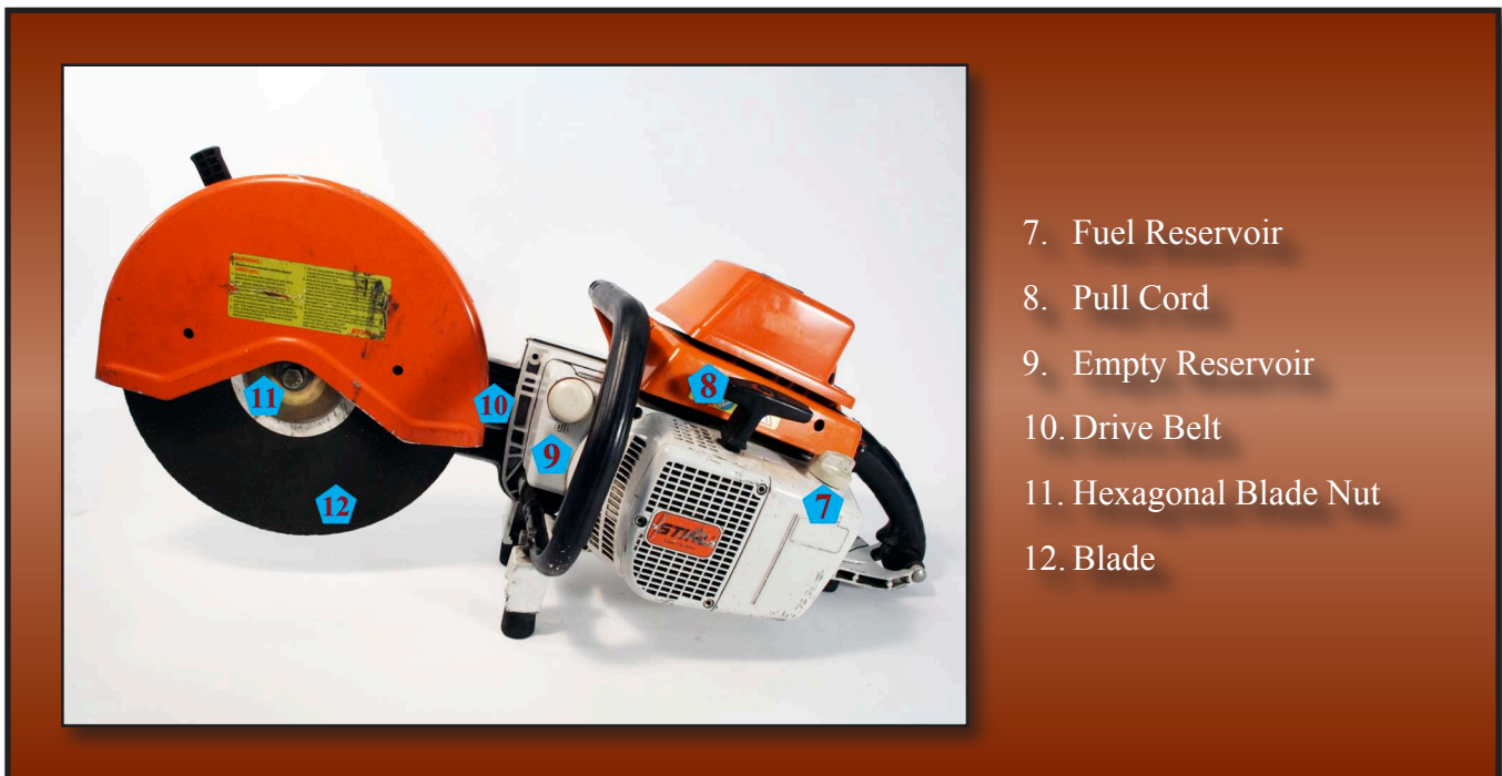
Figure 5-12 Left Side Rescue Saw Schematic
