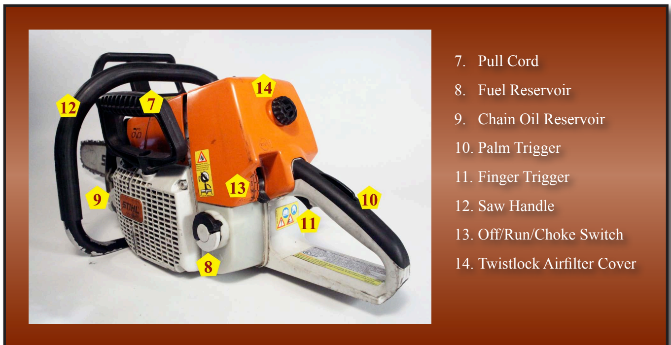
Figure 5-10 Left Side Chainsaw Schematic
