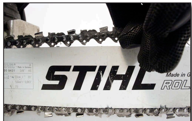
Figure 5-7 Proper Chain Tension
